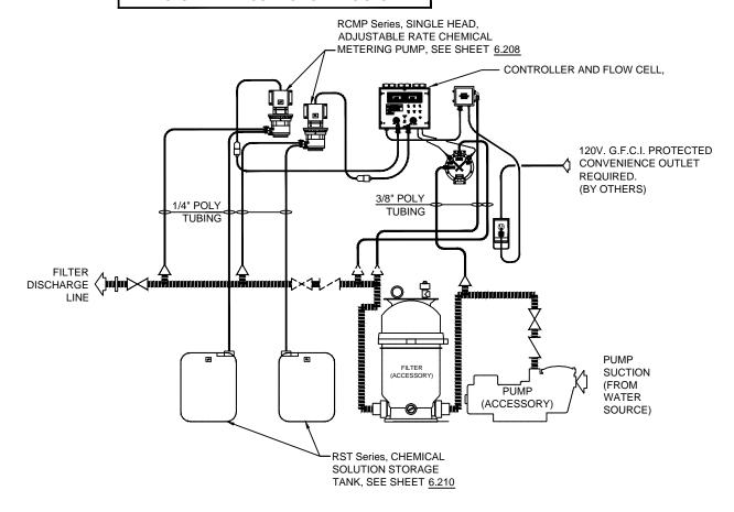
SPECIFICATION DATA: Dual-Point Water Treatment System, for automated maintenance of pool water (pH) and sanitizer (ORP) levels. System consists of: Dual-Point controller with digital read-out, flow cell mixing sampling chamber with clear view cover, ORP and pH electrodes and rotary flow sensor. Metering pump to be installer mounted to wall or tank adjacent to controller. Also includes necessary tubing and compression fittings, and chemical solution tanks.
