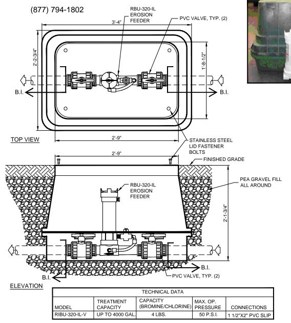
SPECIFICATION DATA: Large capacity 'HDPE', injection molded two-piece plastic housing with re-inforcing ribs, and bolt-down lid. In-line erosion type chemical feeder/sanitizer unit with inlet control valve, threaded lid w/'O' ring gasket, 1 1/2"x 2" socket PVC connectors (reducing bushings included), and two (2) PVC valves for unit service isolation purposes.
