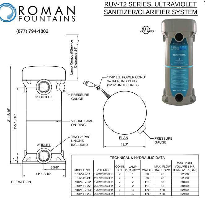
Notes: 1. 230V units are provided with blunt cut cord end only, for hard wiring; plug <u>not</u> included.
