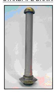
**TECHNICAL DATA** CONNECTION **DIMENSION DIMENSION DIMENSION** MAX. DRAIN MODEL NO. SIZE 'C' RATE 'A' ROV-200-S 2" 3-3/16" 5-5/8" 2-5/16" 50 GPM ROV-300-S 3" 4-3/8" 6-1/2" 3-1/8" 75 GPM ROV-400-S 4" 5-3/4" 7-1/2" 4-1/2" 100 GPM
