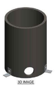
SPECIFICATION DATA: RWD-P Series, PVC Wave Dampener assembly shall consist of Sch. 80 PVC construction and SS anchor tabs. Anchor tabs contain clearance holes for 1/4" anchoring hardware (By Installer).
