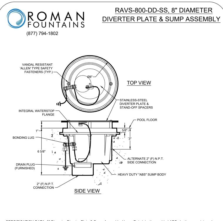
SPECIFICATION DATA: 8" Diameter Diverter Plate & Sump Assembly; Heavy Duty injection molded ABS plastic sump, integral waterstop and 2" (F) N.P.T. side and bottom connections with PVC male threaded plug for un-used connection, 8" diameter Stainless-Steel diverter plate and "ALLEN" type S.S. vandal resistant safety fasteners and wrench.
