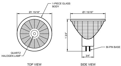
20 WATT, 12V. \_\_\_\_\_ 35 WATT, 12V. \_\_\_\_\_ 50 WATT, 12V. \_\_\_\_
