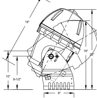
SPECIFICATION DATA: Jumping Jet is constructed of plastic and stainless steel (AISI 304) for use in fresh and pool water; 12V AC; 50Hz; Laminar water jet with cut-off function, selectable RGB-LED light. This unit can be used indoors or outdoors. Must be used with appropriate DMX controller (consult factory).
