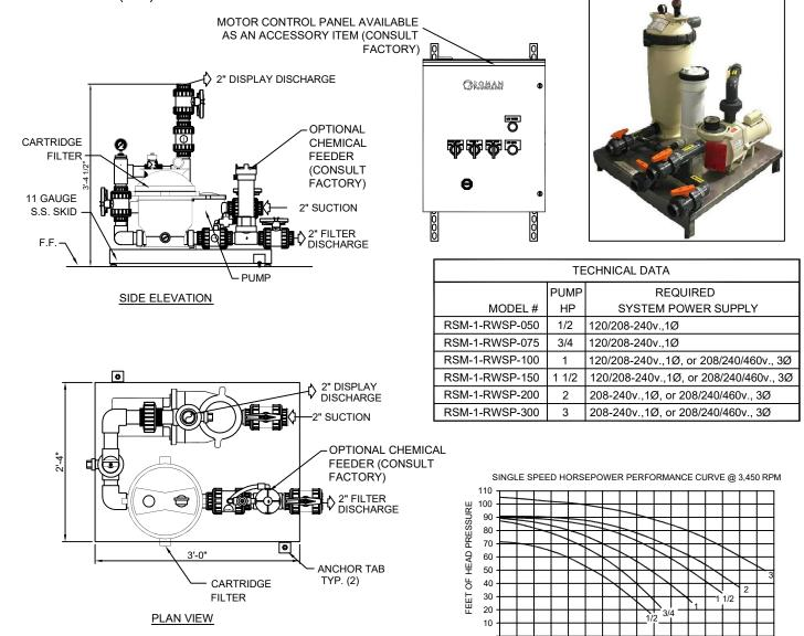
SPECIFICATION DATA: Skid-Mounted Pump/Cartridge Filter Station; consisting of a reinforced 11 gauge, mill finish stainless steel platform with leveling feet measuring approximately 28"W x 36"L, recirculating pump and strainer with the horsepower and power requirement as specified in table above, 50 sq. ft. cartridge filter; necessary isolation and check valves, Schedule 80 PVC piping.
