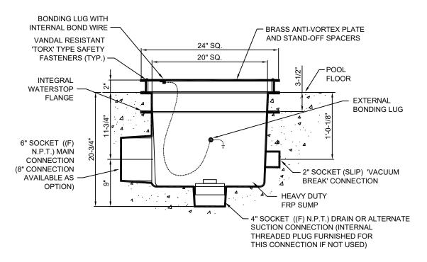
SPECIFICATION DATA: 24" Square Diverter Plate & Sump Assembly; Heavy Duty FRP sump with integral waterstop flange and 6" (socket) side (8" connection available as option), 4" bottom and 2" 'vacuum break' (socket) connections. (the 4" internal connection shall be provided with a 4" threaded male plug). Solid brass 3/16" thick diverter plate with brass spacer, "TORX" type S.S. vandal resistant safety fasteners, and wrench
