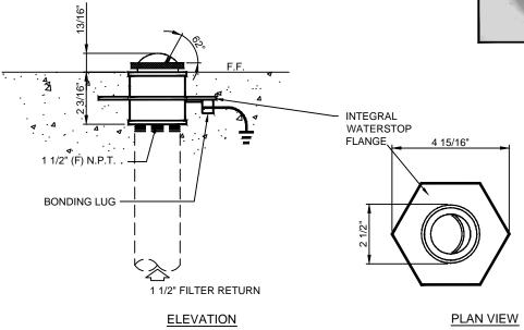
NOTE: INSTALL WATERSTOP FLANGE FACE FLUSH TO FINISHED FLOOR.
