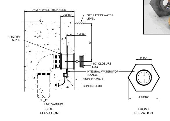
NOTE: INSTALL WATERSTOP FLANGE FACE FLUSH TO FINISHED WALL.
